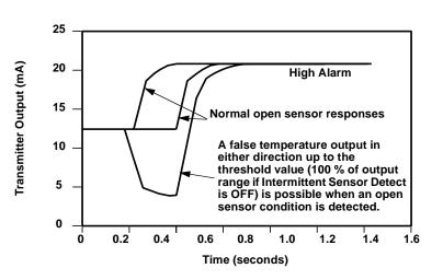
Unless rapid response rate is necessary, the suggested setting of the Intermittent Sensor Detect mechanism is ON.
